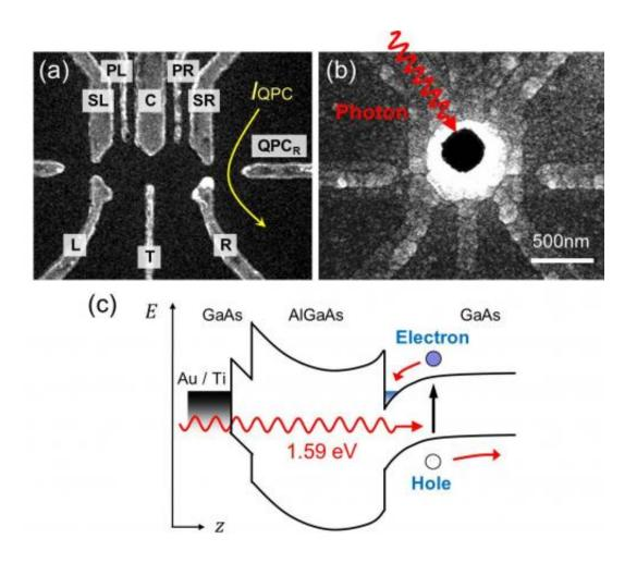
(color online). (a) A scanning electron micrograph of the typical lateral DQD device. The surface gates for dot formation have Tið10 nmÞ=Auð20 nmÞ metal thickness. A 60 nm thick Al2O3 insulating layer was formed on top of them by atomic layer deposition. (b) A Tið30 nmÞ=Auð220 nmÞ mask was fabricated on the surface above the DQD with an aperture of 400 nm diameter. (c) Band
