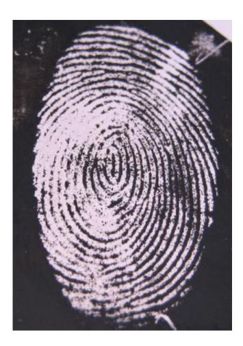
Images of a fingermark left on a stainless steel substrate, following enhancement by electrodeposition of polypyrrole. The light regions are stainless steel that was protected by the sweat residue that was laid on top, preventing the polymer depositing onto it. The dark regions are the polymer in between the fingerprint sweat without the fluorescence 'turned on.' Credit: University of Leicester
