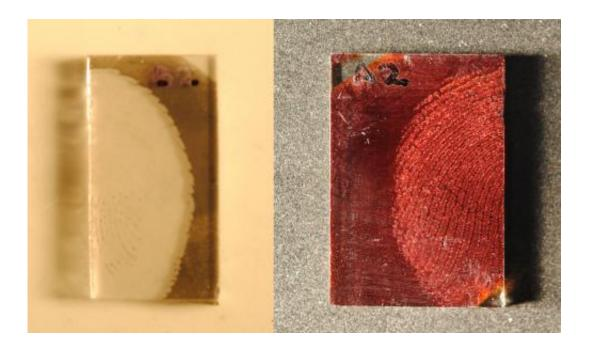
The fingerprint on the left was prepared using an older development technique and does not show much ridge detail. The image on the right was prepared using new CTF technique and shows a lot of ridge detail. Both images are right and left halves of the same fingerprint. Credit: Akhlesh Lakhtakia, Penn State
