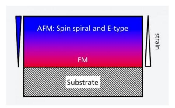
Diagram of the processes in the LuMnO3 layers studied. The layer is especially strained close to the substrate, which leads to a ferromagnetic order there. As the distance grows, the strain decreases so that two antiferromagnetic orders appear: the spin spirals and the E-type, where two spins point in one direction and the next two in the other.
