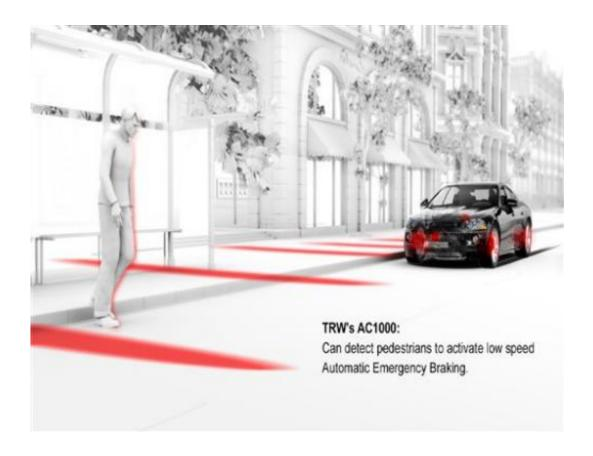
This photo provided by TRW Automotive shows a radar and camera systems that warn you, with beeping sounds, of a possible front-end crash is highlighted. The systems are the outgrowth of adaptive cruise control, which came out 15 years ago and helps keep cars a safe distance from vehicles in front of them. (AP Photo/TRW Automotive)
