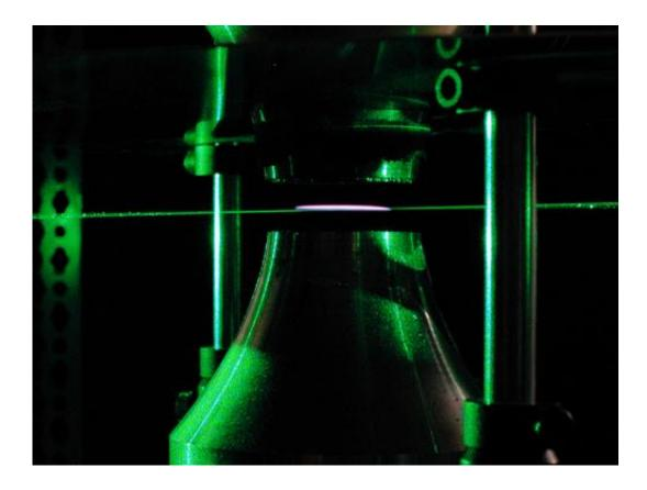
A pulsed laser is used to measure the temperature at the point where a laminar flame is extinguished.Credit: Michael Renfro
