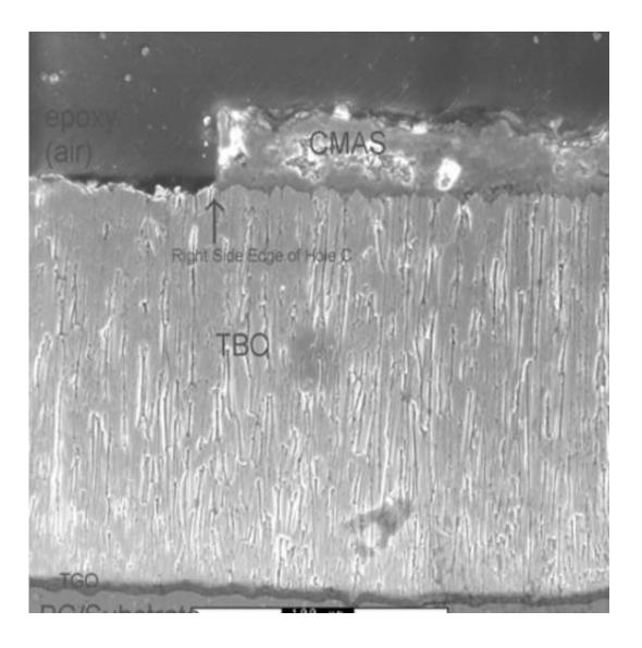
An image showing the successful laser ablation of contaminants from the thermal barrier coating on the surface of a turbine engine blade.Credit: Michael Renfro/Surface & Coatings Technology
