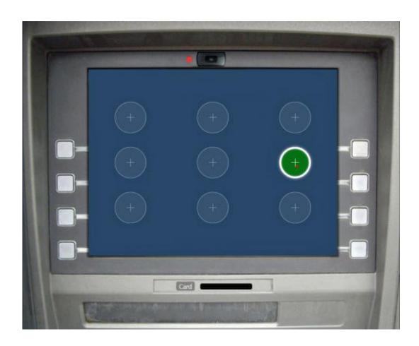
The prototype was built to simulate an ATM screen. In this scenario, users followed the highlighted dots with their eyes and the technology tracked their unique eye movements. Credit: Michael Brooks
