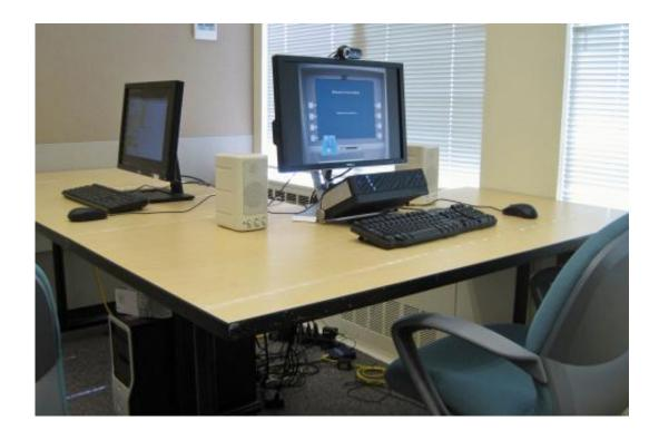
Researchers developed this prototype to test eye-tracking authentication. The monitor shows a welcome screen and the eye tracker is positioned below. Credit: Michael Brooks, U of Wash.
