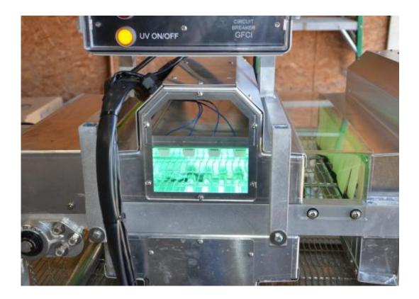
Dr. Craig Coufal's egg sanitizing machine uses a combination of germicidal UV light and a hydrogen peroxide spray to kill bacteria on hatching eggs. Here, an acrylic panel allows the operator to check the condition of the UV lights while blocking any harmful effects. Credit: Texas A&M AgriLife Extension Service photo by Robert Burns
