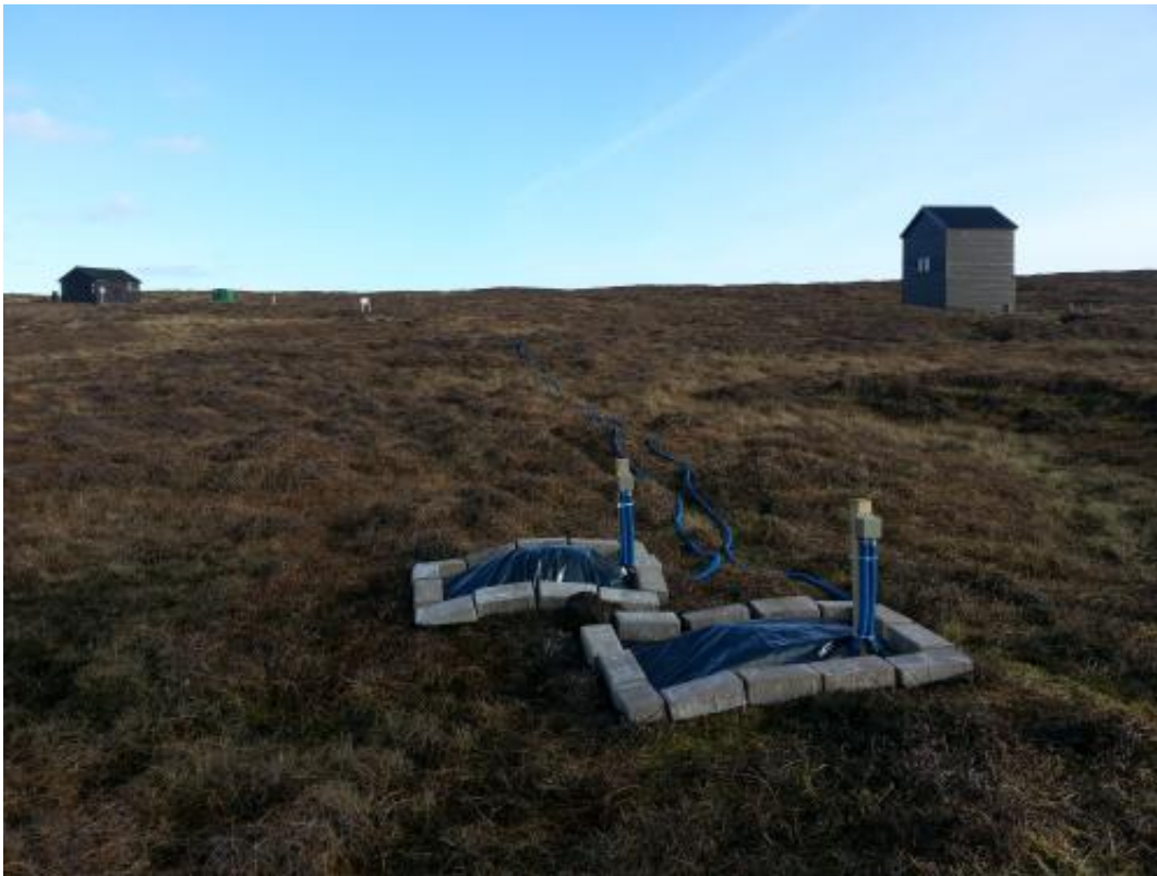
Two of the measurement electrodes at Lerwick observatory in the Shetland Islands. Credit: British Geological Survey, NERC
