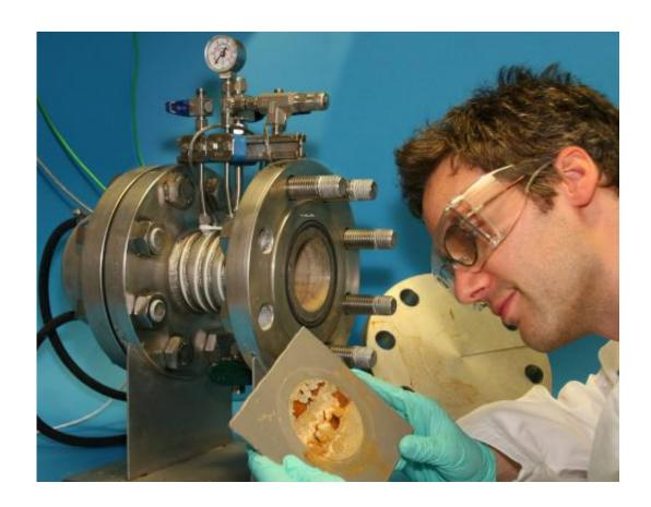
Fitness test failure! Examining a coating sample after a resistance test has been conducted in the Atlas cell. Credit: Fraunhofer IWM
