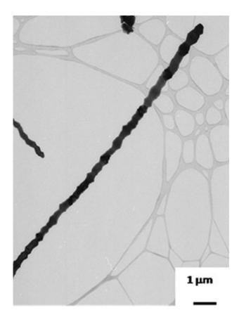
This scanning electron microscope image shows a single wire, tens of thousands of times thinner than a human hair, which was created in a furnace at Ohio State University. Engineers here are growing carpets of these wires on titanium surfaces to boost cell growth, with the ultimate goal of helping the body heal around bone and joint implants. Credit: Image courtesy of Sheikh Akbar, Ohio State University.
