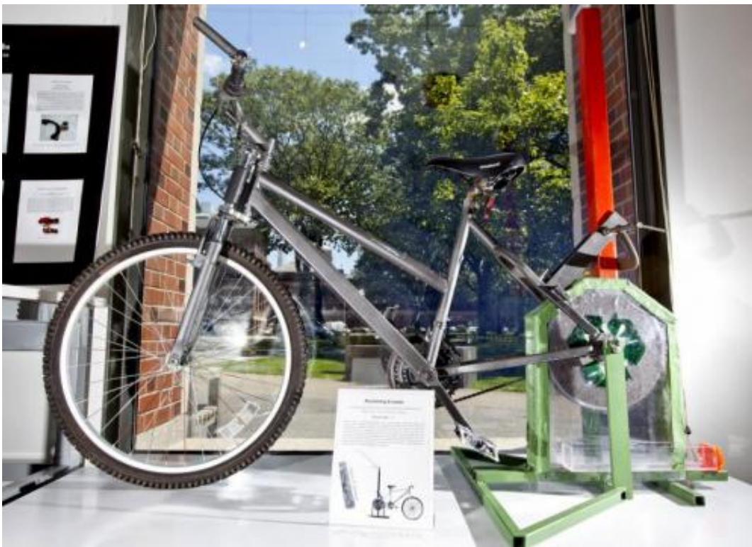
The first prototype of the Bicyclelean replaces the back wheel of a bicycle with a pedal-powered grinding wheel that pulverizes electronic waste. Credit: Eliza Grinnell, SEAS Communications
