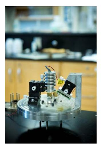
Steven Higgins and his team are building a new version of the hydrothermal atomic force microscope, an instrument that could unlock scientific mysteries and be used in the study of oil production, hydrofracturing of rock layers, storage of radioactive waste and the capture and storage of atmospheric carbon dioxide.
