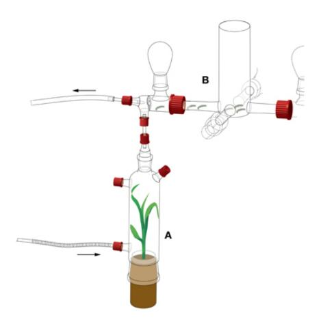
This image shows the detail of the four-arm olfactometer setup for *S. littoralis* larval behavior. Credit: Drawing by Thomas Degen (thomas-degen.ch)
