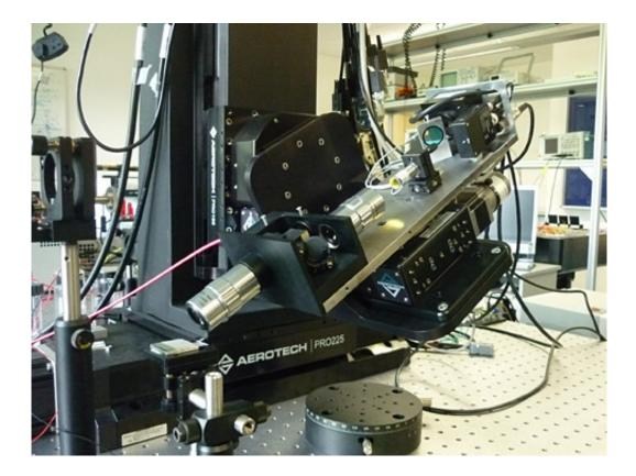
The new optical interferometry system for fast areal surface measurement of microscale and nanoscale surfaces.
