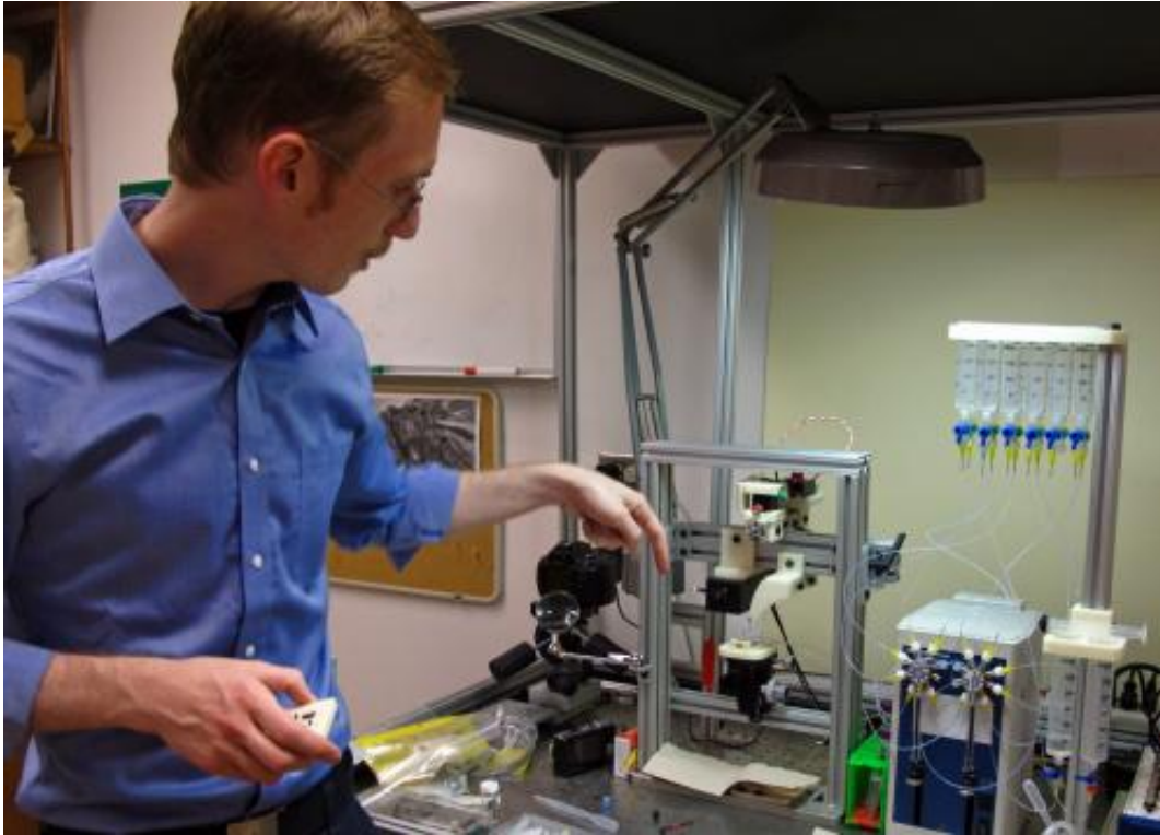
C. David Williams with X-ray diffraction apparatus used to measure lattice spacing of filaments in moth wing muscle samples. Credit: A Kidder
