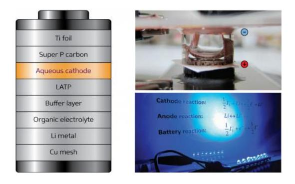
A new type of lithium-ion battery that uses aqueous iodide ions in an aqueous cathode configuration provides twice the energy density of conventional lithium-ion batteries. enlarge image Reproduced from Ref. 1  $\bigcirc$  2013 Y. Zhao et al.
