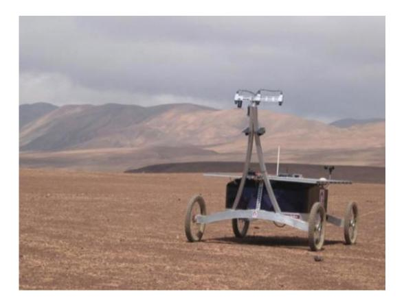
Zoë sets out bravely in the Atacama. Like the Spirit and Opportunity rovers, which landed on Mars in 2004, Zoë is powered by solar panels. Because dust on the panels sometimes shuts down the rovers, the Curiosity rover, which reached Mars in 2012, is nuclear powered. In the Atacama, however, Zoë's panels can be cleaned if they should become dusty. Credit: A. Wang
