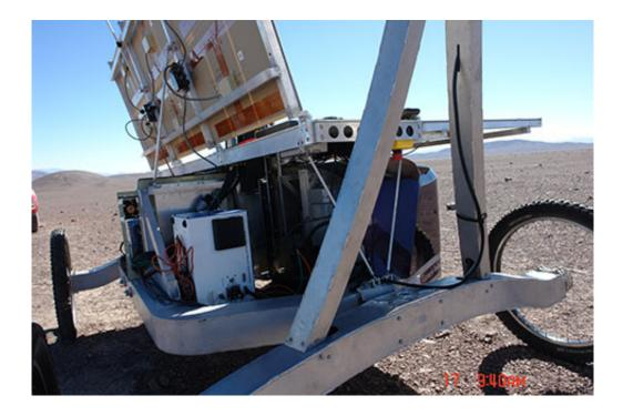
The laser Raman spectrometer (silver box) aboard Zoë. The peaks in a Raman spectra immediately identify the chemical compounds in the sample, without further processing. None of the instruments aboard the rovers currently on Mars
