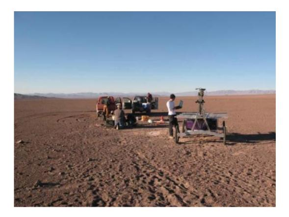
Zoë being checked out at start of the traverse. In the background are the two 4x4 trucks that we will use to follow the robot. The engineers stay within communication range to monitor the robot, but try to say out of view as much as possible. Credit: CMU Field Robotics Center
