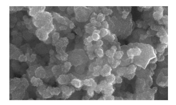
These copper zinc tin sulfide nanoparticles help form a solar cell that could cost less and perform well. Credit: Oregon State University
