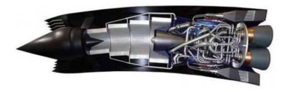
A cutaway view of the proposed Sabre engine, which is being developed by Oxfordshire-based Reaction Engines. Credit: Reaction Engines
