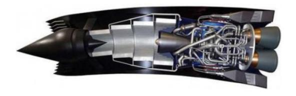
A cutaway view of the proposed Sabre engine, which is being developed by Oxfordshire-based Reaction Engines. Credit: Reaction Engines
