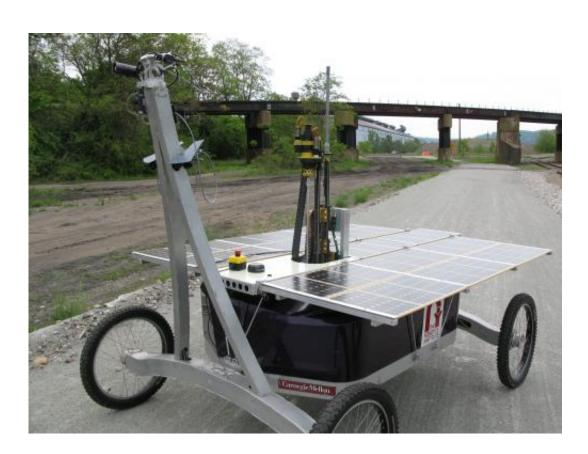
The Zoe robot will use a one-meter drill, shown here protruding above the robot's solar cell deck, to search for subsurface life in Chile's Atacama Desert. Carnegie Mellon University's Robotics Institute and the SETI Institute are leading the NASA-sponsored field experiment. Credit: Carnegie Mellon University
