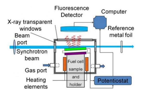
Schematic of the custom-designed furnace used to test solid-state fuel cell components in action at beamline X18B at the National Synchrotron Light Source.
