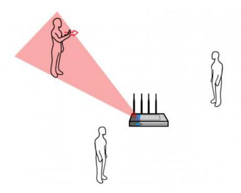
WiSee technology uses multiple antennas to focus on one user to detect the person's gesture.
