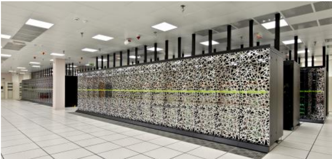
Fig. 1: For its simulations the MPA team uses supercomputers that belong to the most powerful in the world. (a) CURIE of the TGCC-CEA computer center with 77,184 processor cores and a nominal peak performance of 1.667 Petaflop/s (1 Petaflop = 1 million billion flops). Credit: GENCI/TGCC-CEA (b) SuperMUC of the Leibniz computing center with more than 155,000 processor cores and a nominal peak performance of over 3 Petaflop/s. Credit: LRZ 2012
