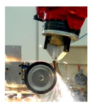
A robot automatically restores the damaged sections of a turbine blade at a grinding station. Credit: Fraunhofer IWF TU Berlin
