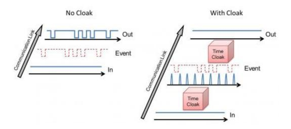
This diagram depicts the basic operation of a "temporal cloak" for optical communications that represents a potential tool to thwart would-be eavesdroppers and improve security for telecommunications. The signal is modified to have zero intensity when the data are "on," cloaking the information. Then the cloak converts the pulses back to a flat signal, hiding the fact that any data were transmitted. Credit: Joseph Lukens, Purdue University
