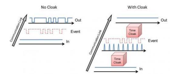
This diagram depicts the basic operation of a "temporal cloak" for optical communications that represents a potential tool to thwart would-be eavesdroppers and improve security for telecommunications. The signal is modified to have zero intensity when the data are "on," cloaking the information. Then the cloak converts the pulses back to a flat signal, hiding the fact that any data were transmitted. Credit: Joseph Lukens, Purdue University
