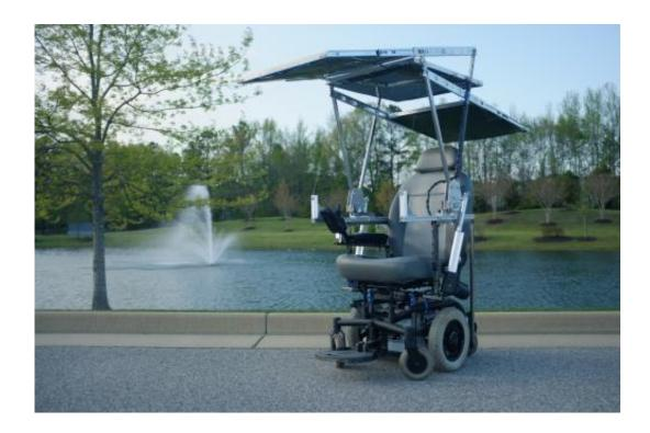
The team's solar-powered wheelchair includes solar panels that are easily deployed and stored, providing nearly unlimited range at low speeds.
