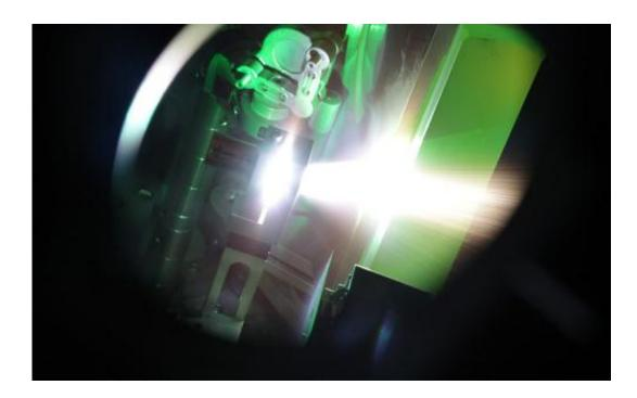
A burst of laser energy 50 times greater than the worldwide output of electrical power slams into an extremely thin foil target to produce neutrons at Los Alamos National Laboratory's TRIDENT laser facility during a recent experiment, which proved that laser-driven neutrons can be used to detect and interdict smuggled nuclear materials. Credit: Los Alamos National Laboratory
