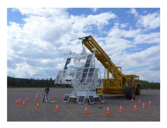
For outdoor tests on 29. May, 2013, the solar observatory Sunrise is held up by the launching vehicle. During the launch, this vehicle will hold Sunrise until the helium balloon is positioned directly above the observatory. Credits: MPS
