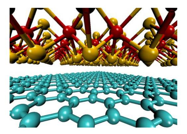
The MIT team found that an effective solar cell could be made from a stack of two one-molecule-thick materials: Graphene (a one-atom-thick sheet of carbon atoms, shown at bottom in blue) and molybdenum disulfide (above, with molybdenum atoms shown in red and sulfur in yellow). The two sheets together are thousands of times thinner than conventional silicon solar cells. Credit: JEFFREY GROSSMAN AND MARCO BERNARDI
