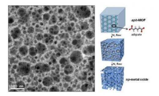
(Left)It shows TEM image of np-MgO-500. (Right) This is the schematic view of the direct conversion from aph-MOG to np-metal oxide by heating under nitrogen atmosphere. Credit: UNIST
