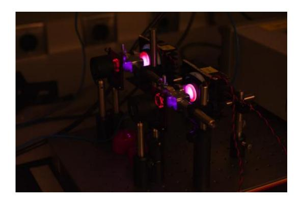
This device tests the quality and reliability of the silicon nanoparticle phosphors that LumiSands created to use in LED lighting. Credit: Mary Levin, UW
