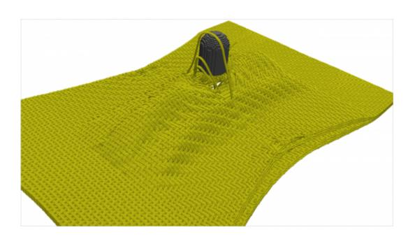
This simulation models the perforation of a six-layer harness satin weave Kevlar target (four inches in width) by a 0.44 caliber copper projectile. Credit: Eric Fahrenthold, The University of Texas at Austin
