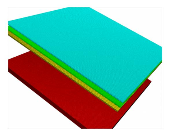
This figure shows a computational model of the spacecraft shielding and wall depicted above. The wall of the spacecraft is shown in red. The shielding is modeled as five layers: aluminum (in yellow), multilayer insulation (in green), and Beta-cloth plus aluminized Mylar (in blue). The model reproduces exactly the correct material areal densities, but the layer count is reduced, in order to reduce computational cost.
