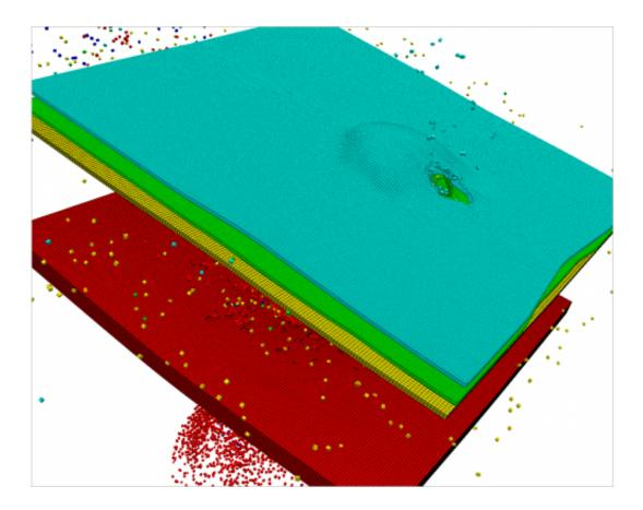
This figure shows simulation results for the impact of a 0.24 cm diameter aluminum projectile on the spacecraft shield and wall depicted above. Impact velocity is 9 km/s and the impact obliquity is 30 degrees. The simulation indicates that this projectile will pass through the shielding system and perforate the wall of the spacecraft.
