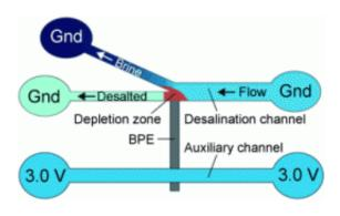
(Phys.org) —A new method for the desalination of sea water has been reported by a team of American and German researchers in the journal *Angewandte Chemie*. In contrast to conventional methods, this technique consumes little energy and is very simple. This electrochemically mediated seawater desalination is based on a system of microchannels and a bipolar electrode.
