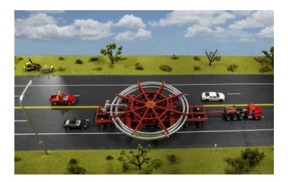
A model of the truck that will be used to transport the Muon g-2 ring, placed on a streetscape for scale. The truck will be escorted by police and other vehicles when it moves from Brookhaven National Laboratory in New York to a barge, and then from the barge to Fermi National Accelerator Laboratory in Illinois. Credit: Fermilab
