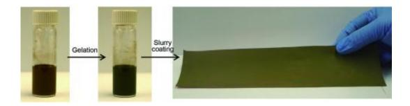
Stanford scientists used a battery fabrication process to make novel silicon/hydrogel electrodes. Silicon nanoparticles were dispersed in a red hydrogel solution, forming a dark-green gel that was bladed onto a copper foil current collector and dried. Credit: Yi Cui, Stanford University
