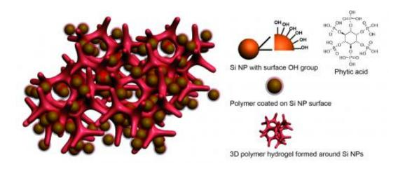
This is an illustration of a new battery electrode made from a composite of hydrogel and silicon nanoparticles (Si NP). Each Si NP is encapsulated in a conductive polymer surface coating and connected to a three-dimensional hydrogel framework. Credit: Yi Cui, Stanford University
