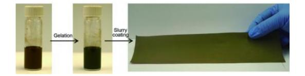
Stanford scientists used a battery fabrication process to make novel silicon/hydrogel electrodes. Silicon nanoparticles were dispersed in a red hydrogel solution, forming a dark-green gel that was bladed onto a copper foil current collector and dried. Credit: Yi Cui, Stanford University
