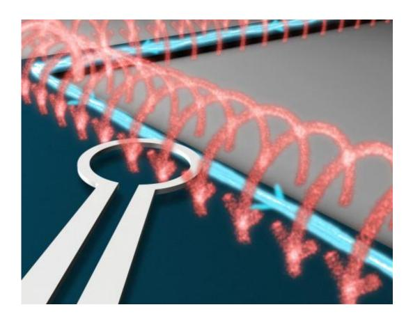
This graphic depicts the tiny loop of a scanning SQUID, or superconducting quantum interference device (silver), which detects magnetic fields (red) created by an edge current (blue) in a topological insulator. Credit: Greg Stewart
