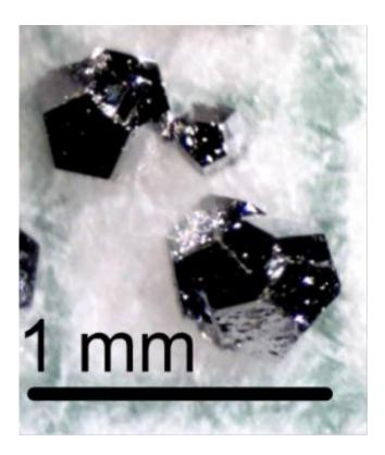
The pentagonal dodecahedral morphology of the icosahedral phase is shown with a millimeter scale; grains as large as 1.0 mm have been grown. Credit: Ames Laboratory, USDOE
