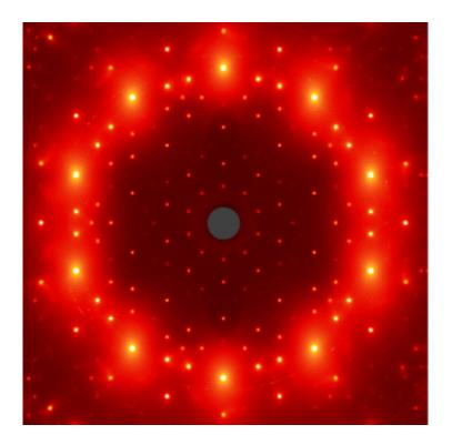
High-energy x-ray diffraction patterns from a single grain of i-Gd-Cd were taken at the Advanced Photon Source at Argonne National Laboratory with the beam parallel to the five-fold axis. Credit: Ames Laboratory, USDOE
