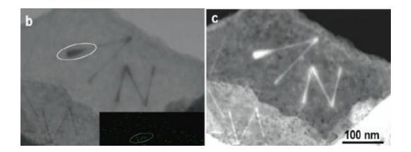
Images taken by a scanning transmission electron microscope (STEM) of electron ink on graphene paper, showing the letter "N" and the symbol " $\Lambda$ ." Credit: Wei Zhang, et al. ©2013 IOP Publishing Ltd.
