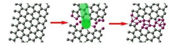
When an electron beam (green) writes on graphene paper, some of the carbon atoms in the graphene are kicked off, and external carbon atoms are deposited onto the dangling bonds to form an irregular structure that appears as "ink." Credit: Wei Zhang, et al. ©2013 IOP Publishing Ltd.
