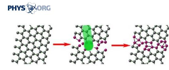
When an electron beam (green) writes on graphene paper, some of the carbon atoms in the graphene are kicked off, and external carbon atoms are deposited onto the dangling bonds to form an irregular structure that appears as "ink." Credit: Wei Zhang, et al. ©2013 IOP Publishing Ltd.
