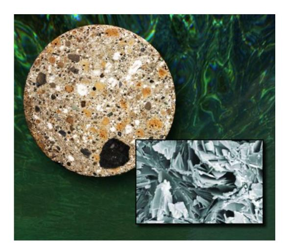
This image shows a drill core of volcanic ash-hydrated lime mortar from the ancient port of Baiae in Pozzuloi Bay. Yellowish inclusions are pumice, dark stony fragments are lava, gray areas consist of other volcanic crystalline materials, and white spots are lime. The inset is a scanning electron microscope image of the special Al-tobermorite crystals that are key to the superior quality of Roman seawater concrete. Credit: Lawrence Berkeley National Laboratory
