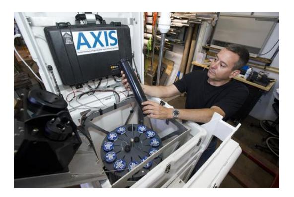
Scientist David Fratantoni led the project to develop the Autonomous eXpendable Instrument System (AXIS), which features a carousel that can store and deploy up to 12 data-collecting probes. Credit: Tom Kleindinst, Woods Hole Oceanographic Institution
