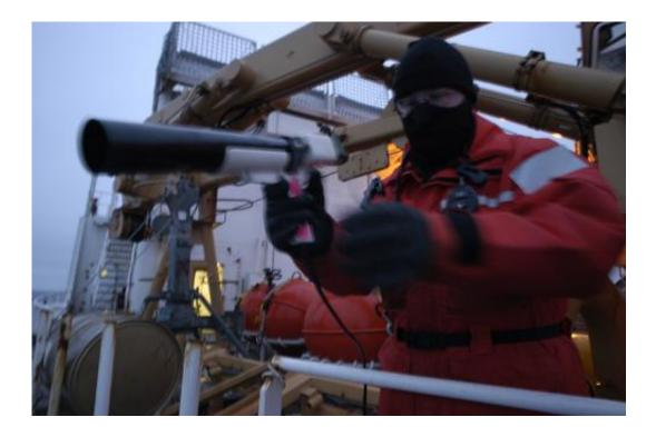
eXpendable BathyThermograph (XBT) probes usually are deployed by hand once per hour over 36 hours, but AXIS will automate the deployment thereby making data collection at sea more efficient and reliable. Credit: Chris Linder, Woods Hole Oceanographic Institution
