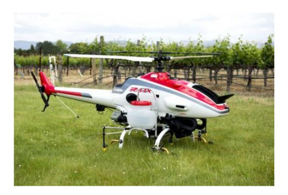
UC Davis researchers test a remote-controlled helicopter to spray pesticides on vineyards, which are normally sprayed using ground vehicles. Yamaha, who supplies Japanese rice farmers with flying sprayers, provided the helicopter for these tests. Photos taken at the UC Davis Oakville Station in Oakville, Ca. on May 7, 2013. Credit: Joe Proudman/UC Davis
