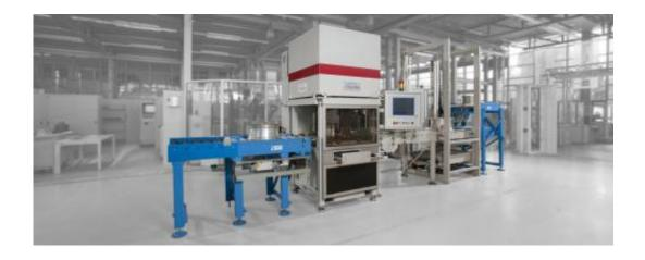
The "Wheelinspector" makes non-contact measurement of light-alloy wheels directly in the production process possible for the first time. Credit: Fraunhofer-Institut für Fabrikbetrieb und -automatisierung IFF
