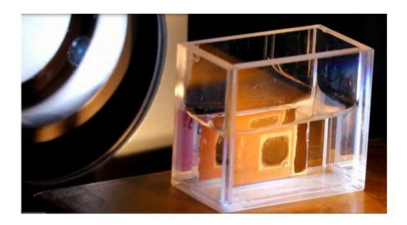
This complex solar cell is coated with two different catalysts and works like an "artificial leaf", using sunlight to split water and yield hydrogen gas. Credit: HZB
