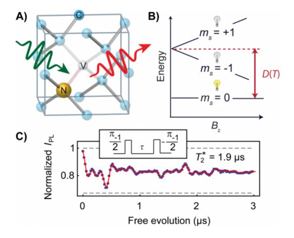
Nitrogen vacancy center in diamond. (A) Depiction of a nitrogen vacancy (NV) center in the diamond lattice. The wavy green arrow represents the 532-nm laser used for optical excitation and the wavy red arrow represents the phonon-broadened fluorescence used to measure the spin state. (B) Fine structure of the NV center ground state as a function of axial magnetic field. The light bulbs represent the relative fluorescence difference for the ms = 0 and ms =  $\pm 1$  states.
