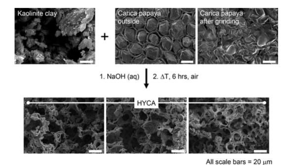
An inexpensive new material made of clay and papaya seeds removes harmful metals from water and could lower the cost of providing clean water to millions of people in the developing world, scientists are reporting. Their study on this "hybrid clay" appears in the journal ACS Sustainable Chemistry & Engineering.
