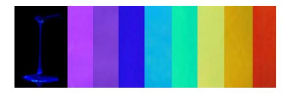
Full-colour luminescence panels under ultraviolet (365nm) irradiation by adjustment of the nonvolatile blue-emitting anthracene liquid (left: photo) in the material.
