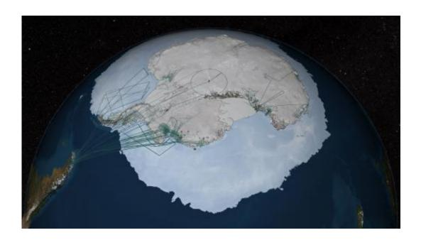
A significant portion of the data in Bedmap2 was collected by NASA's Operation IceBridge. Flight paths from the 2009, 2010 and 2011 Antarctic campaigns are shown here as dark green lines. NASA DC-8 flights originated from Punta Arenas, Chile, on the left side of the image. Flight lines in East Antarctica represent surveys flown by the Institute for Geophysics at the University of Texas at Austin, one of IceBridge's partnering organizations. Credit: NASA Goddard's Scientific Visualization Studio
