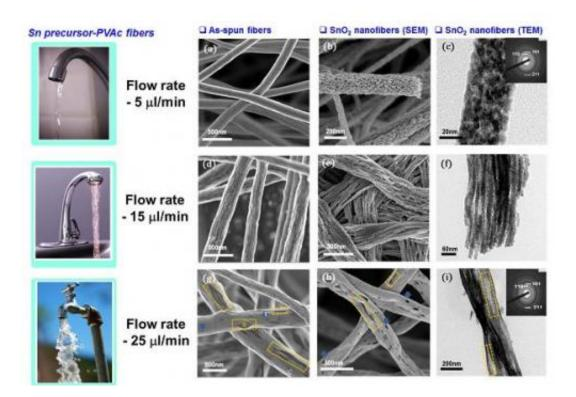
This is the microstructural evolution of SnO2 nanofibers as a function of flow rate during electrospinning. Credit: KAIST
