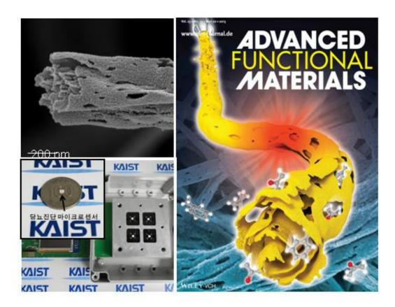
Clockwise from left to right: left upper shows a magnified SEM image of a broken thin-wall assembled SnO2 fiber. Left below is an array of breath sensors (Inset is an actual size of a breath sensor). The right is the cover of *Advanced Functional Materials* (May 20th issue) in which a research paper on the development of a highly sensitive exhaled breath sensor by using SnO2 fibers is published. Credit: KAIST
