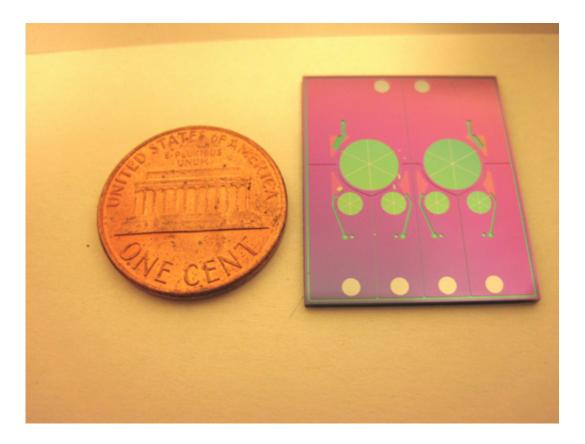
Researchers at the University of Michigan developed three different pumps in three different pressure categories. From lowest to highest pressure, the categories are microplasma Penning ion high vacuum, Knudsen mid vacuum, and high-frequency peristaltic rough vacuum pumps. Pictured above is a 24-stage microscale rough pump that uses tiny micromachined hexagonal compartments, where each element of the array is either a pump or a valve.
