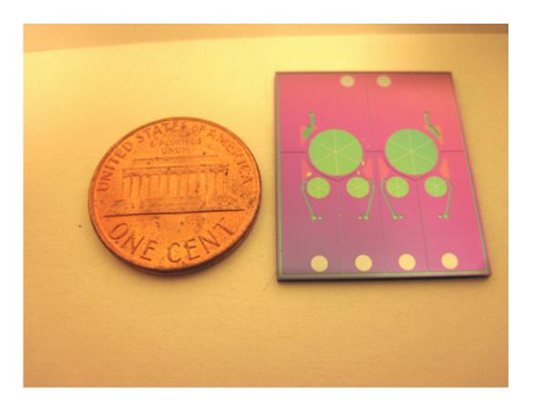
Researchers at the University of Michigan developed three different pumps in three different pressure categories. From lowest to highest pressure, the categories are microplasma Penning ion high vacuum, Knudsen mid vacuum, and high-frequency peristaltic rough vacuum pumps. Pictured above is a 24-stage microscale rough pump that uses tiny micromachined hexagonal compartments, where each element of the array is either a pump or a valve.
